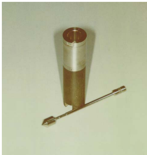
Figure 1: Brookfield SC4-14 spindle with the 6R small sample adapter
